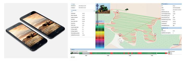
Data collection is automatically done by data loggers. All data generated in real time can be seen on the ODOKUS website and on mobile terminals. The real-time data provide all necessary information to control harvesting processes, for coordinating liquid manure logistics and for general monitoring of your fleet.
