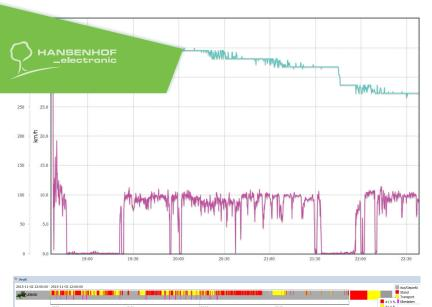
The alert system automatically sends messages if defined limit values are exceeded or fallen short of (operating life, velocity, geo-fencing, machine and device parameters).
